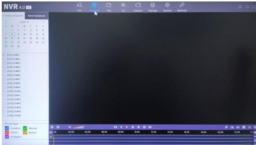
2. „Smart playback” – Acest meniu permite cautarea si redarea inteligenta a inregistrarilor in functie de cautarile efectuate dupa camera si tip de eveniment: Motion event, Humanoid event, Eelectronic fence, Cross-boundary, Off-duty detection, Passenger flow
