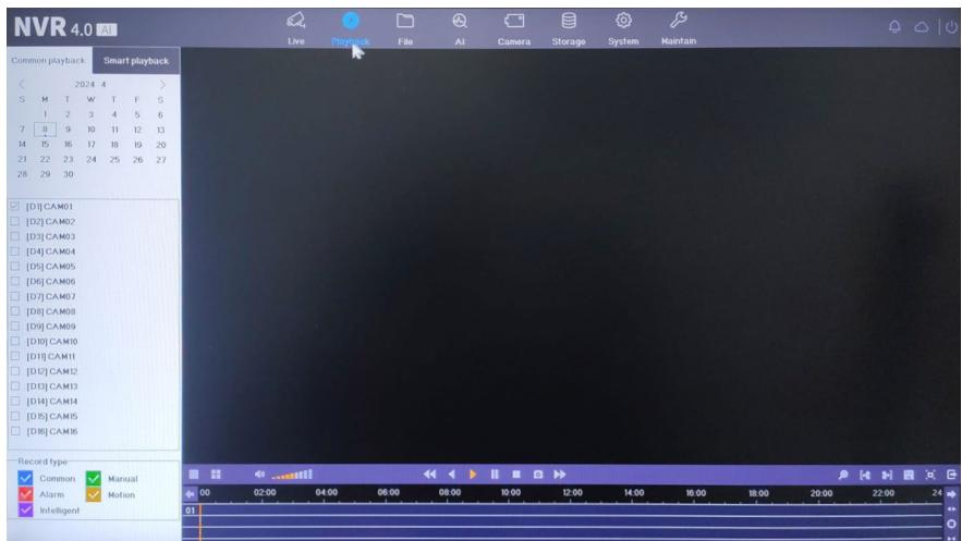
"Smart playback" – This menu allows searching and intelligent playback of recordings depending on the searches performed by camera and type of event: Motion event, Humanoid event, Electronic fence, Cross-boundary, Off-duty detection, Passenger flow.
